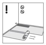
Important: installation with foil to the bottom
